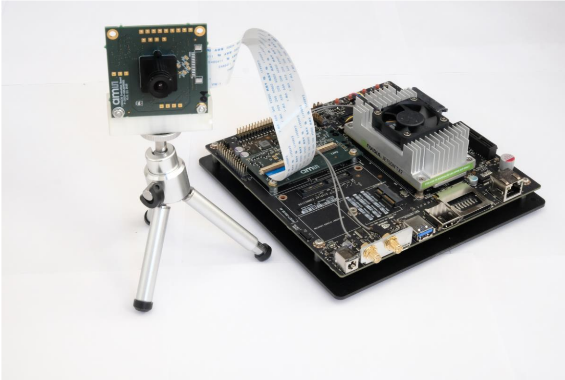
AMS demo kit with NIR-enhanced sensor combined with a NIR light source
