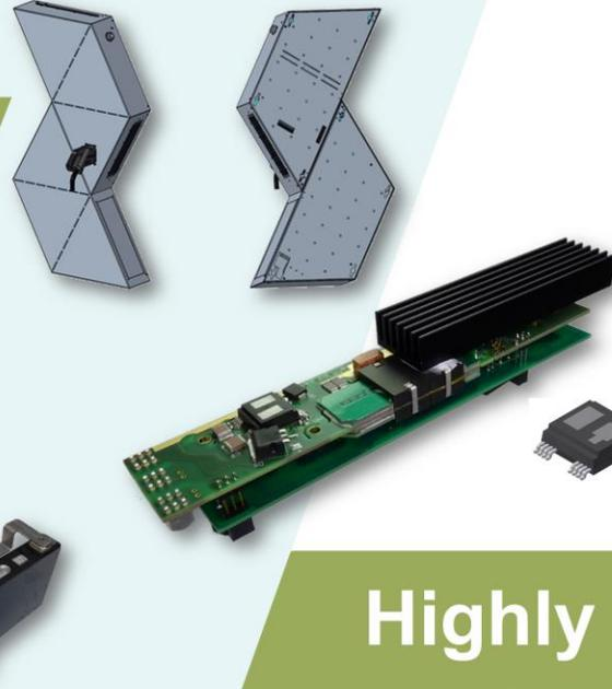
Two stage converter design to fulfill isolation requirements and charging standards with Bidirectional power transfer to enable storage capability of renewable energies
